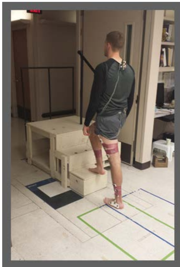
Figure 38: Motion capture set-up for stair-climb analysis with left foot on the force plate and right taking the first step up.
